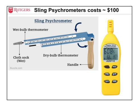
• Sling Psychrometers are cost effective way of determining on-site wet-bulb temp. You need to wet the clock sock on the wet bulb thermometer and then sling it for few minutes.
