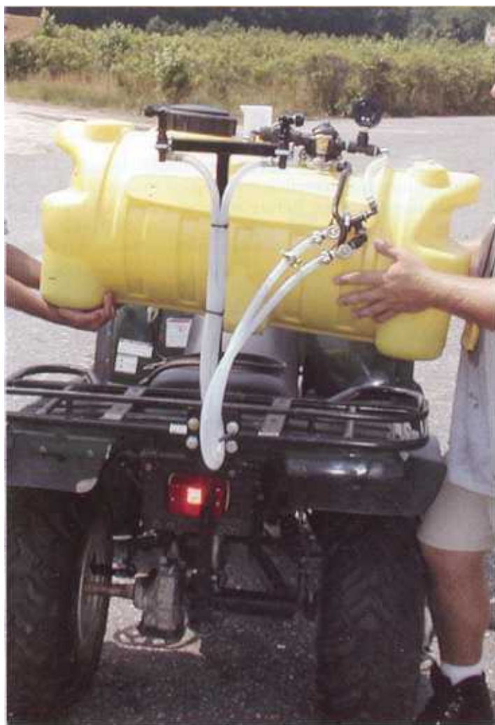
Figure 9. Low gallonage sprayer setup on 4-track for spinosad bait sprays.
