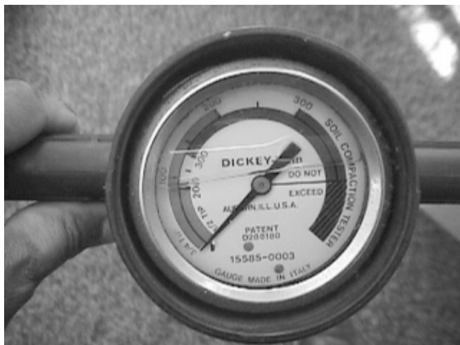
Read-out dial of penetrometer Photos by Ray Samulis
