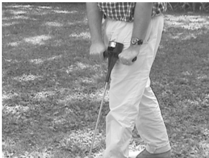
Measuring soil compaction with penetrometer
