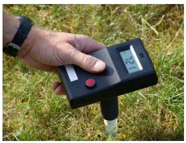
newer Tensiometer with data logger
