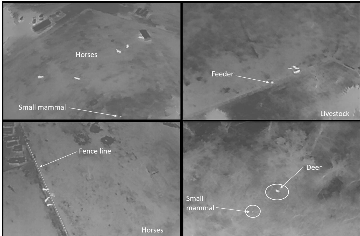
Figure 17: Examples of how different objects and animal species have unique thermal signatures that are utilized for species identification during drone surveys.
